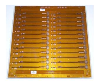
Flexible circuit array bonded to a pre-routed FR4 carrier panel. Circuits are easily removed after assembly.
